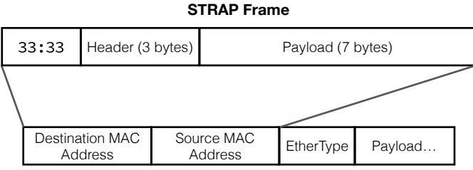
Fig. 2: The composition of a STRAP frame and how it fits in an Ethernet frame.
