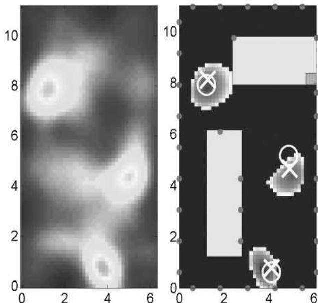
**Figure 1: On the left, the original RT image formed by the system when three people are located in the monitored area. On the right, the RT image after being processed by the machine vision methods used to track multiple people. The dots represent the radio transceivers, the white circles the true position of people, the white crosses their estimated position, and the grey rectangles furniture present in the area.**
