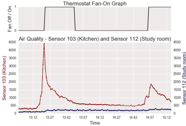
**Figure 1: (Bottom) PM2.5 sensor value for UMDS in kitchen (red) and study room (blue); and (Top) furnace fan state. The fan is triggered by, and then helps to reduce, the high pollutant level in the kitchen, but its use marginally increases pollution in the study room.**
